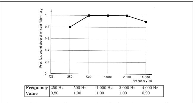
Figure 1 — Reference curve for evaluation of weighted sound absorption coefficient,  $\alpha_{\rm w}$
