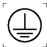
Figure 5 – Symbol IEC 60417-5019: Protective earth
